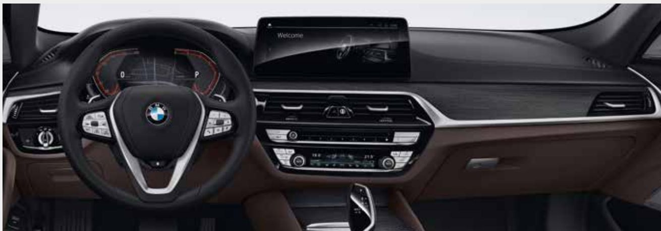
The newly developed interface design of BMW Live Cockpit Professional with Navigation makes using the infotainment system in the BMW 5 Series easier, more lucid and intuitive. The 31 cm (12.3") LCD display has Touch Functionality, configurable home screen, 3D Maps and can also be operated through iDrive Touch Controller, and Voice Control.
